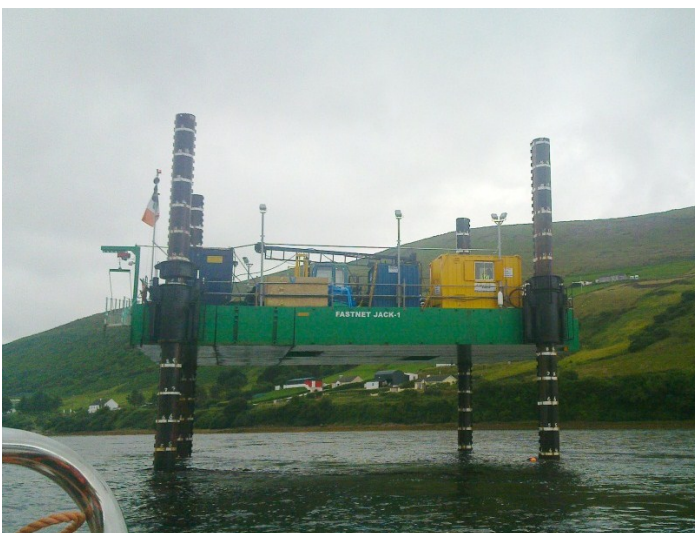
** Pictures depict the combifloat units used in Self Elevating Platform Mode**
